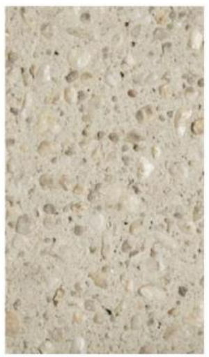
In-situ decorative surfacing etch and aggregate finishes ranging from the 0.5mm (left) to approx. 3mm (right)
